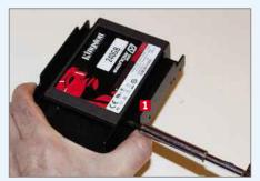
To install an SSD in a desktop PC, you'll need a 2.5in to 3.5in adapter. Your new drive may come with one but, if it doesn't, you can pick one up for around £7 from the likes of Amazon. Ground yourself to disperse any static electricity, as in Step 1, then insert the SSD into the adapter and screw it in. 11
