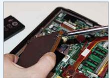
Laptop hard drives are the same size as SSDs, so you simply swap one for the other. Remove the battery from the laptop, ground yourself on a radiator or similar, and remove the back of the case. Take out the old hard drive and replace it with the new SSD, then attach the power and SATA connectors and reassemble everything.
